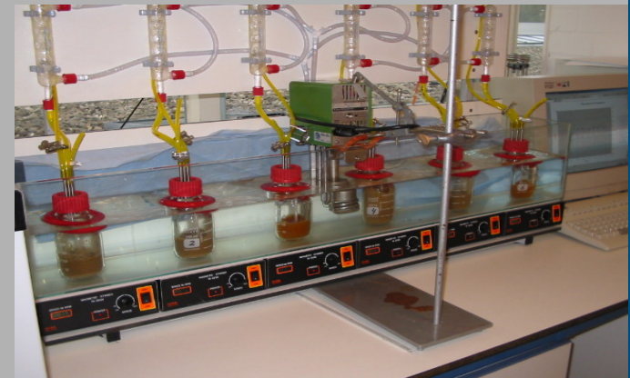
Bench-scale fermentation with on-line CO 2 monitoring
